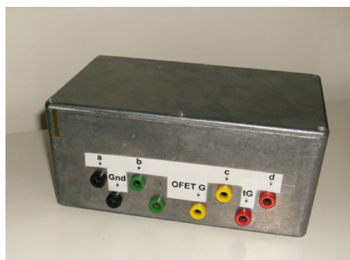
FIG. 2. (Color online) A picture of the metal box used for shielding the sample and eliminating the effect of light during I-V measurement.
